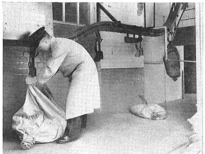
FIG. 6—CHAIN-CONVEYOR LOADING POINT AT LEAMINGTON SPA SORTING OFFICE
