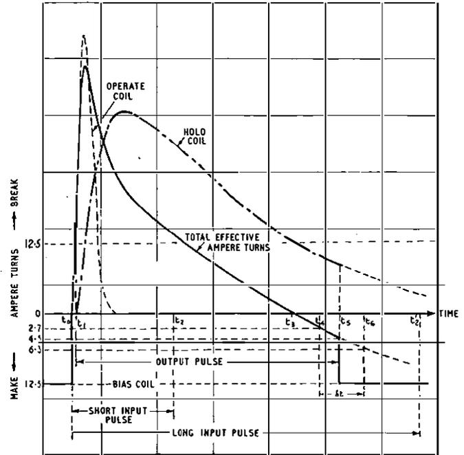
FIG. 8.—VARIATIONS OF AMPERE-TURNS DURING ONE CYCLE.
