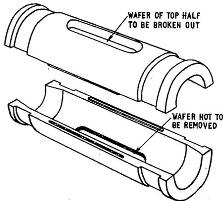
FIG. 3.—WATER-BARRIER COUPLING.
