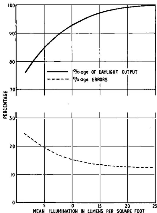
Note: Daylight illumination during the test was of the order of 100 lumens/ft².
