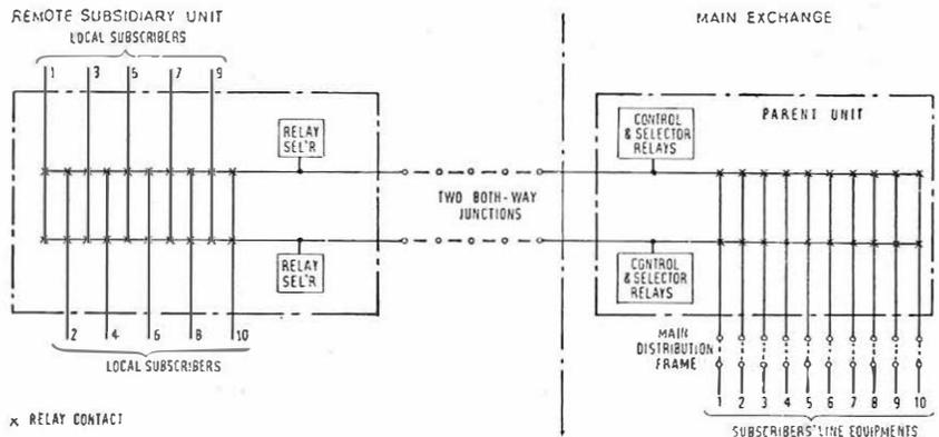
A call at either end of the system causes the selecting relays to hunt. The corresponding outlets at each end of the junction are selected simultaneously and tested for *calling* and *busy* conditions. When the calling condition is located the hunt action is arrested, and interconnection between the subscriber and the subscribers' line equipment is provided by the junction. The call then proceeds in the normal manner according to the type of Parent Exchange.
