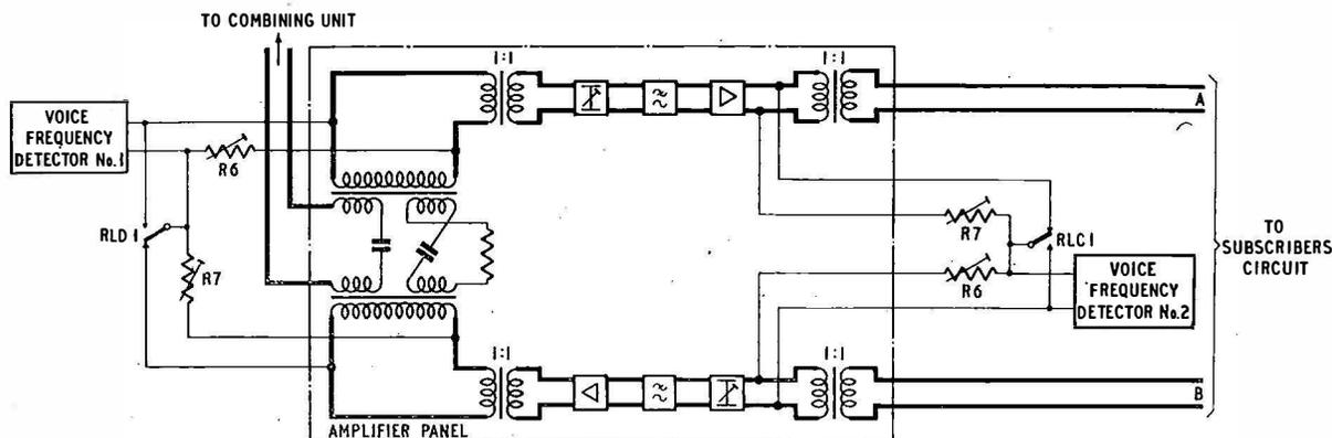
Notes 1. Relay RLC operates when signals enter detector No. 1 and relay RLD operates when signals enter detector No. 2.
