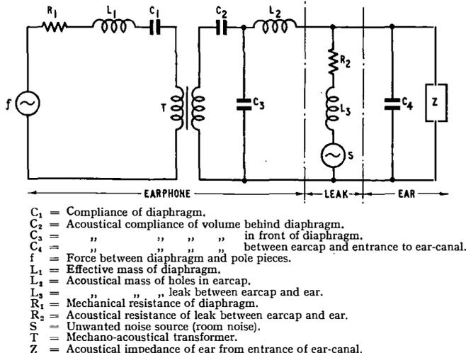
FIG. 3.—SIMPLIFIED ANALOGOUS ELECTRICAL CIRCUIT OF EARPHONE AND EAR.
