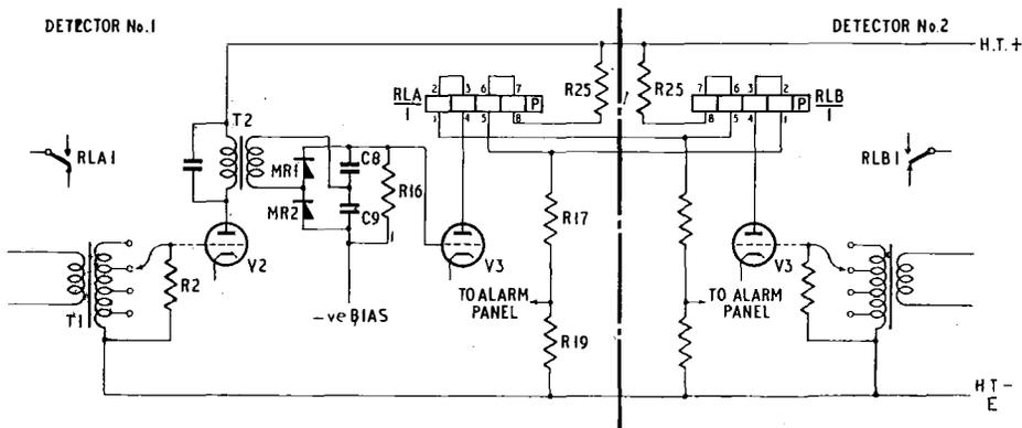
Note. The cathodes of valves V3 are connected to the bridge circuits on the control panel (see Fig. 5)
