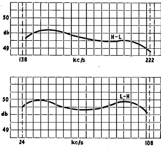
FIG. 16.—TYPICAL REPEATER CONVERSION GAIN/FREQUENCY RESPONSE.
