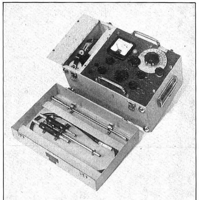
FIG. 2.—RECEIVER, RADIO, NO. 12 (30 TO 100 Mc/s).
