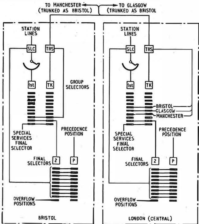
SLC = Station Line Circuit. TRS = Trunk Relay Set. P = Precedence Final Selector.
