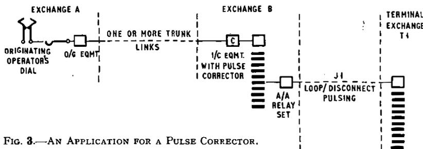
FIG. 3.—AN APPLICATION FOR A PULSE CORRECTOR.
