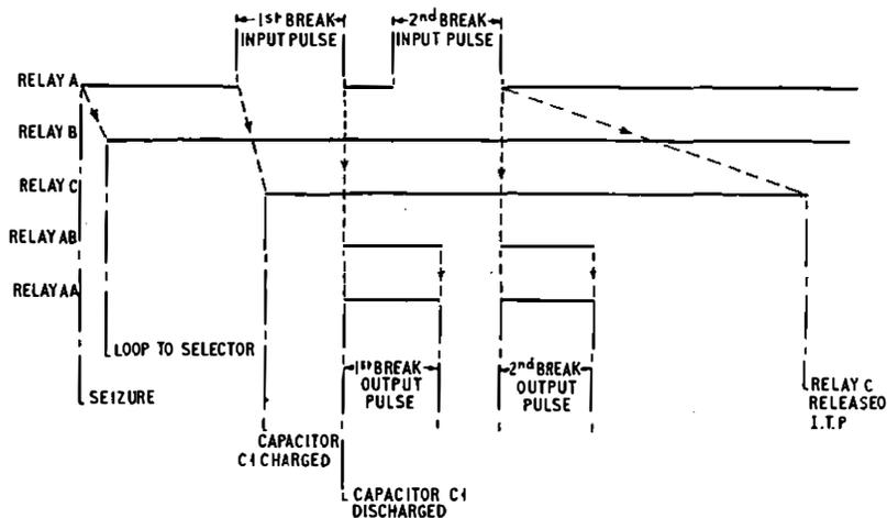
Note.—An arrow points to the relay which is energized or de-energized by the operation or release of the relay from which the arrow starts.
