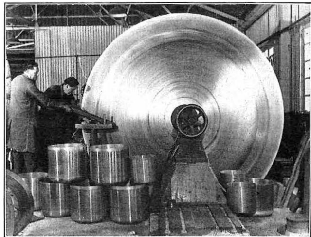
FIG. 12.—SPINNING A 12-FT DISH.
