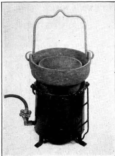
FIG. 3.—GAS FURNACE AND PLUMBER'S POT.
