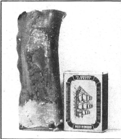
DAMAGE DONE TO CABLE SHEATH BY DORMOUSE.
