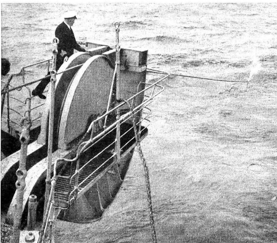
FIG. 9.—CABLE PAY-OUT OVER THE STERN SHEAVE.
