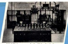
200-kW long-wave single-sideband telephony transmitter at Rugby, 1926
