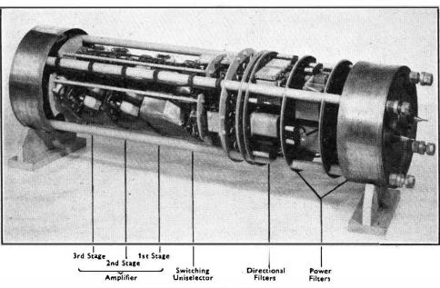
FIG. 11.—EARLY SUBMERGED TELEPHONE REPEATER.
