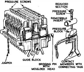
FIG. 15.—SKETCH OF ASSEMBLY STRIP.
