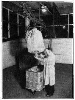
FIG. 4.—BAG OPENING FROM A CHAIN CONVEYOR.
