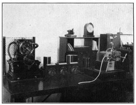
FIG. 5.—BAUDOT DISTRIBUTOR AND RECEIVER.
