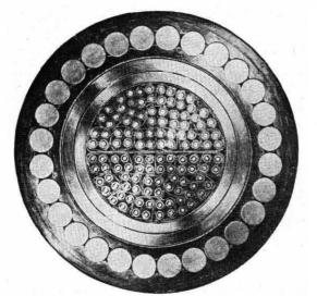
Fig. **6**.—Cross-section of Anglo-Belgian Cable of 1932 (actual size).
