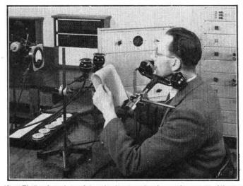
Note: The list of speech sounds is speken into the microphone under test; one of the two high-quality microphones and the level meter are used for controlling the loudness of speaking.
