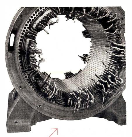
A parily wound stator for a 13,000 h.p. motor.
