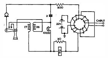
Note: Principal component t pes are: (a) Receiver, similar to Western Electric Company (W.E.) T pe 2657A; (b) Transmitter, solid back with No. 7 Button, similar to W.E. Type 2617A; (c) Induction coil, similar to W.E. Type 2203; (d) Supervisory relay, similar to W.B. Type 1007P; (e) Re ting coil, similar to W.E. No. 25C.
