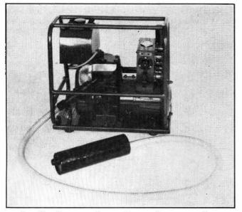
FIG. 14.—PORTABLE ENGINE-DRIVEN GENERATING SET.
