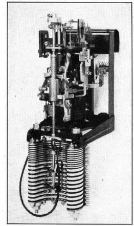
FIG. 5.—AN EARLY TWO-MOTION SWITCH (SIEMENS BROS.).
