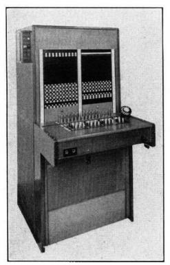
FIG. 18.—MODERN LAMP-SIGNALLING SWITCHBOARD (P.M.B.X. No. 1A).
