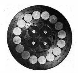
FIG. 4.—CROSS-SECTION OF A 4-CORE CROSS-CHANNEL CABLE LAID IN 1910 (ACTUAL SIZE).
