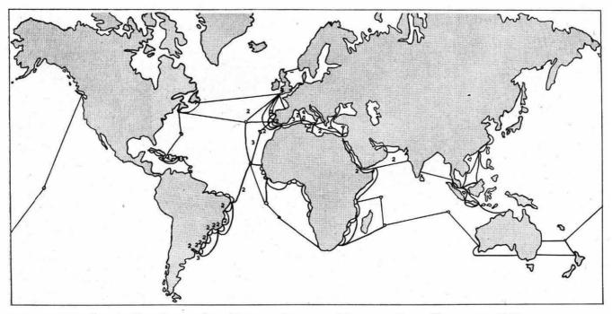
FIG. 1.—THE BRITISH LONG-DISTANCE SUBMARINE TELEGRAFH CABLE NETWORK IN 1906.
