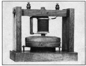
FIG. 1.—A REPLICA OF GRAHAM BELL'S ORIGINAL TELEPHONE.
