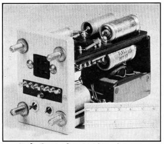
FIG. 9.-NEGATIVE IMPEDANCE AUDIO AMPLIFIER.
