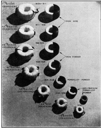
Photograph by Standard Telephones & Cables Ltd. FIG. 1.—LOADING COILS, FROM 1900 TO 1956.
