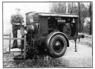
FIG. 11.-MODERN POWER-DRIVEN WINCH.
