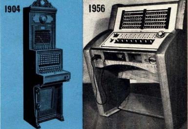
A very early type of G.E.C. manual switchboard—a few of these boards are still in operation to-day—and (right) the modern G.E.C. press-button switchboard on the Royal Yacht.
