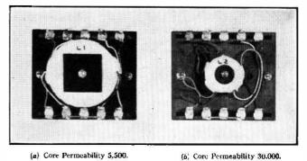
FIG. 13.—REDUCTION IN SIZE OF WIDE-BAND TRANSFORMERS BY THE USE OF HIGH-PERMEABILITY CORE MATERIALS.
