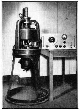
FIG. 2.—THE FRANCKE A.C. GENERATOR AND A MODERN AUDIO-FREQUENCY TEST OSCILLATOR.
