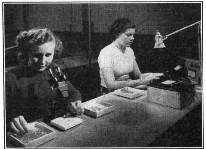
FIG. 7.—FINAL INSPECTION OF 1A THERMISTORS.
