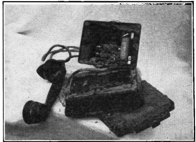
SUBSCRIBER'S INSTRUMENT AFTER PENETRATION BY SAND.
