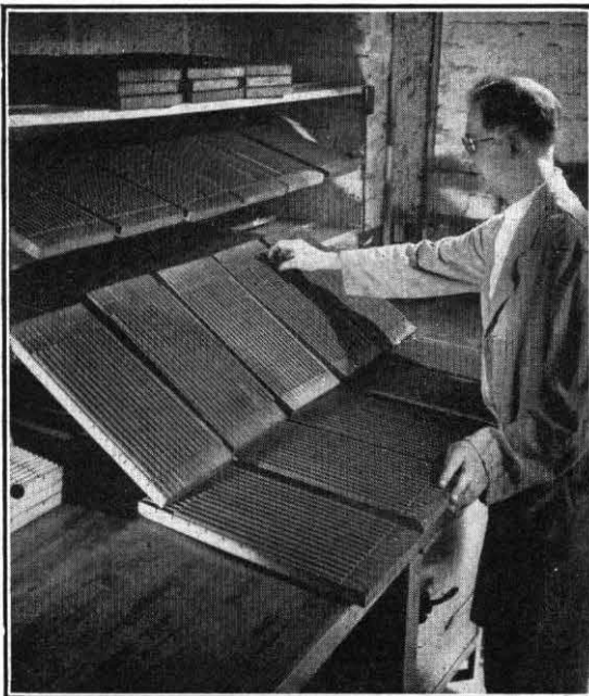
FIG. 2.—TRAYS OF BRIMISTOR MATERIAL AFTER CURING.
