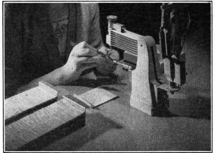
FIG. 6.—WELDING WIRES OF 1A THERMISTOR TO A CUNIFE HAIRPIN.
