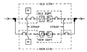
Fig. 2.—Connections at Existing Station before New Equipment is Cut In.
