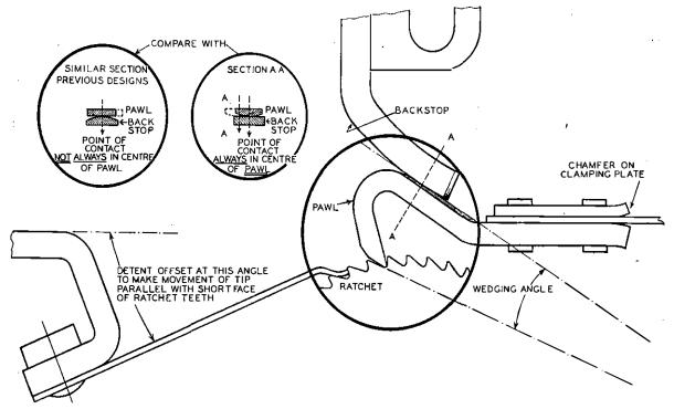
Fig. 5.—Main Features of Driving Mechanism.
