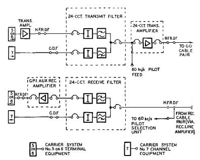
Fig. 8.—Utilisation of Carrier System No. 5 or 6 Terminal Equipment FOR GROUP 1, AND No. 7 CHANNEL EQUIPMENT FOR GROUP 2.
