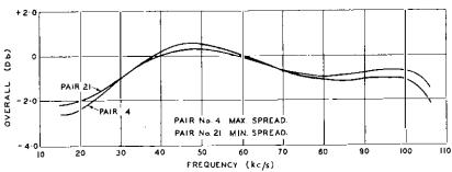
FIG. 5.—MAXIMUM AND MINIMUM VARIATIONS OF LEVEL WITH FREQUENCY ON LONDON-LEICESTER SECTION OF LONDON-DERBY NO. 2 CABLE,
