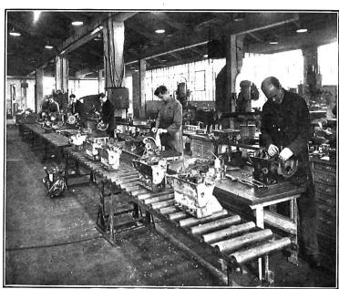
Fig. 5.—Engine Assembly Line.
