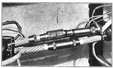
Fig. 5.—Construction of Joints in 0.975 Inch Tubes.
