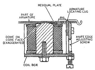
Fig. 4 — Cross-Section of Coil Box and Armature.
