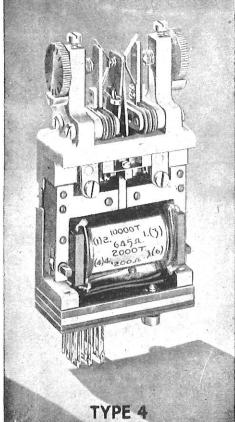
This is a medium speed, sensitive relay with long contact travel designed primarily as a telephone impulsing relay (D.C. dialling up to 100 miles and V.F. dialling on trunk circuits). It has also been successfully adopted for use in Telex systems.
