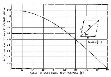
Fig. 2.—Ratio of Magnitude of Sum of Two Equal Voltages at Angle  $\theta^{\circ}$ , to Magnitude of a Single Voltage.
