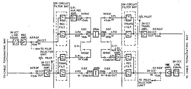
Fig. 9.—Group 1 Made Available and Group 2 Connected Through,
