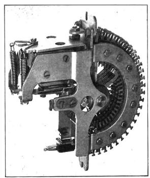
Fig. 1.—P.O. Uniselector Type 2—5 Level.
