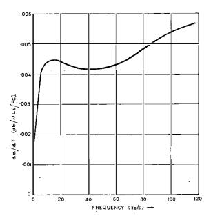
FIG. 6.—CABLE P.C.Q. CARRIER 12-QUAD 40-LB. SIDE CIRCUIT. VARIATION OF ATTENUATION (a) WITH TEMPERATURE (T) (DB./MILE/°C) V. FREQUENCY.
