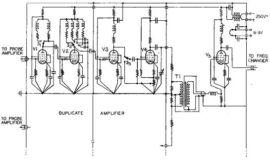
Fig. 3.—"Twin" Amplifiers Circuit.
