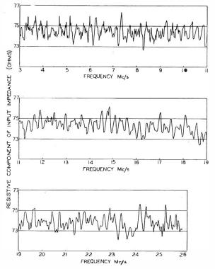
Fig. 8.—Variation of Resistive Component of Input Impedance with Frequency for 3-Mile Length of 0.975
