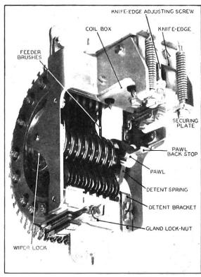
Fig. 2.—P.O. Uniselector Type 2—8 Level.
