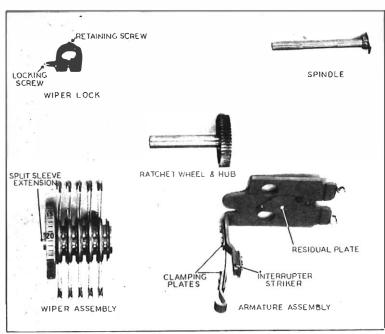
Fig. 6.—Parts of Uniselector Type 2.
