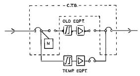
Fig. 3.—Existing Equipment Replaced by Temporary Equipment.
