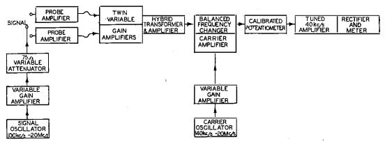
Fig. 1.—Block Schematic Diagram of Phase Meter.
