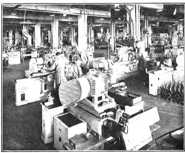
Fig. 3.—Crankshaft Grinders.
