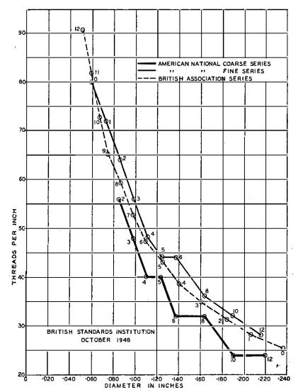
Fig. 3.—Comparison Between British and American Standard sizes For Theads In The Range Below  $\frac{1}{4}$  inch.
