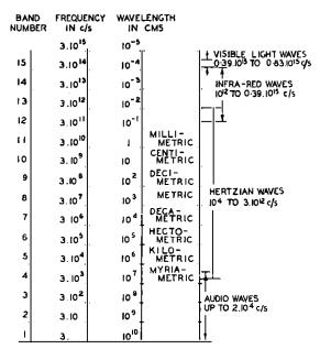
Fig. 1.—Frequency and Wavelength Ranges Corresponding to Proposed Band Numbers.
