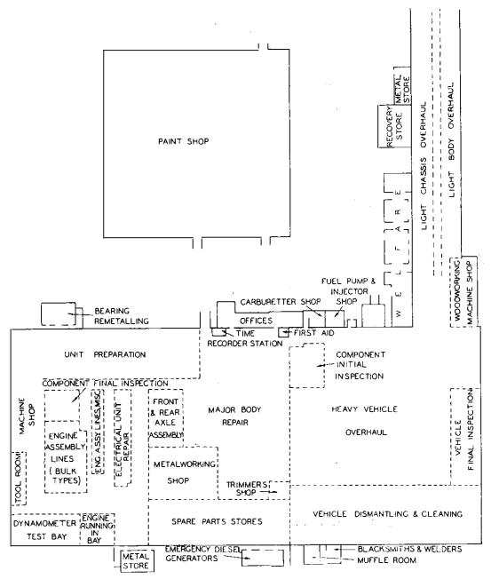
FIG. 1.—LAYOUT OF YEADING REPAIR DEPOT.
