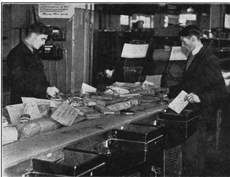
FIG. 1.—HAND-STAMPING TABLE WITH CHUTES.
