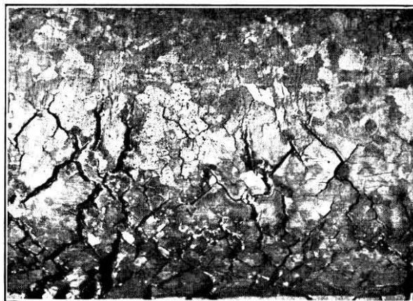
FIG. 2.—FATIGUE CRACKS DUE TO LARGE CRYSTALS (MAG. \times 5 ).
