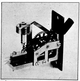
FIG. 1.--MECHANISM OF DELAYED ACTION KEY.
