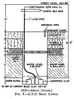
manner shown in Fig. 7, which also illustrates the strata and general scheme. The resistance of this combination measured  $2.5 \Omega$  on completion.
