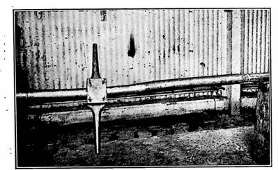
FIG. 5.—SWAGE CLAMPED TO CABLE.
