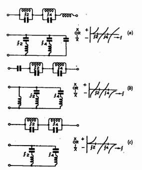
FIG. 3.—REACTANCE AND SUSCEPTANCE CURVES OF VARIOUS CIRCUITS
