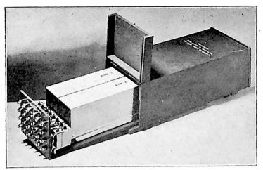
FIG. 5 .- BALANCE AND BY-PASS UNIT.
