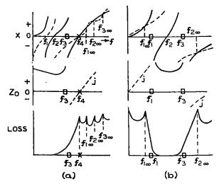
FIG. 7.-LOW PASS AND BAND PASS FILTER CURVES.
