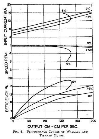
efficiency-output power curves are shown in Fig. 4. It will be seen that with a battery voltage of  $7\frac{1}{2}$  V and with an output of about 100 gm. cm. per second a change in battery voltage of  $\pm 20$  per cent. produces a change in speed of less than  $\pm 1$  per cent. The relatively high efficiency of the motor can also be seen from the curves.
