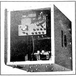
FIG. 2.-RECTIFIER WITH TOP COVER REMOVED.
