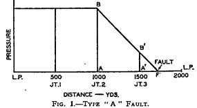
The pressure in one half section remains steady, proving that section to be sound, and in the other half Joint 3 shows a lower figure, and the far end, nil.
