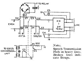
FIG. 1.—OPERATION OF RINGER IN 2-WIRE LINE.
