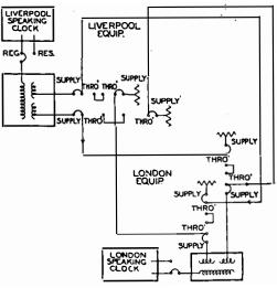
FIG. 2.—OMNIBUS TRUNK CIRCUIT CONNECTIONS AT REPEATER STATIONS.
