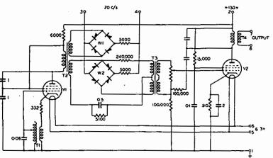
FIG. 4.-500 C/S OSCILLATOR WITH STATIC "CHOPPER."
