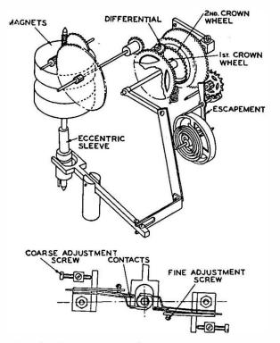
Fig. 6.—Constructional Details of Experimental Motor.
