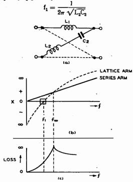
FIG. 2 .-- REACTANCE AND LOSS CURVES FOR A SIMPLE LOW-PASS LATTICE FILTER NETWORK.
