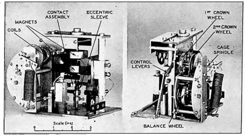
FIG. 5.-EXPERIMENTAL IMPULSE MOTOR.
