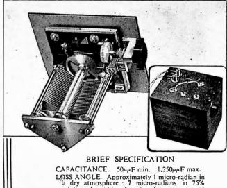
LOSS ANGLE. Approximately 1 micro-radian in "a dry atmosphere: 7 micro-radians in 75% relative humidity, for the frequency range 50 c.p.s. to 10,000 c.p.s. DRIVE. Worm reduction gear, 50 : 1 ratio. SCALE READING. To 1 part in 5,000 direct reading; To 1 part in 20,000 by interpolation. BACKLASH. Not exceeding 1 part in 20,000. DIMENSIONS. 127 x 10 x 131.
