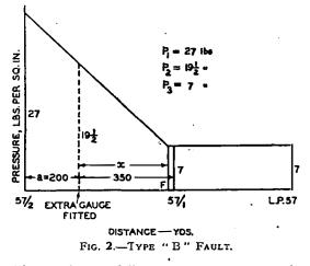
After 3 hours, full pressure was measured at LP 58, and only 6 lb. at LP 57. The fault thus lay between LP 57 and the mid-point, 57/2. A measurement at 57/1 showed 7 lb. From this it was not clear whether the fault lay between 57 and 57/1, or between 57/1 and 57/2, although the latter appeared to be the case. After a further hour, 57/1 and 57 both showed 7 lb.; in other words, equalisa-
