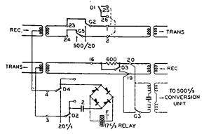
FIG. 2.—OPERATION OF RINGER IN 4-WIRE LINE.
