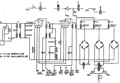
FIG. 3.-500/20 c/s CONVERSION CIRCUIT.
