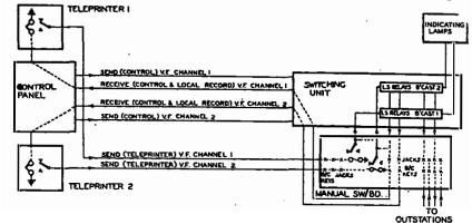
FIG. 3.—SCHEMATIC DIAGRAM OF TELEPRINTER BROADCAST SYSTEM.
