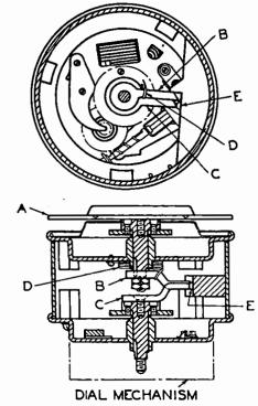
FIG. 5.—DIAL MECHANISM FITTED WITH SLIPPING CLUTCH DEVICE.
