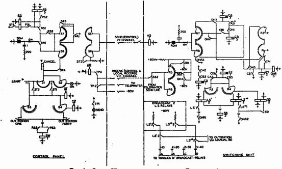
FIG. 4.—CIRCUIT ELEMENTS ASSOCIATED WITH BROADCAST 1.
