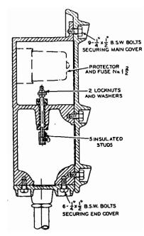
FIG. 7. PROTECTOR AND FUSE UNIT.
