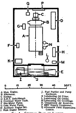
FIG. 1. GENERAL PLAN OF LAYOUT.
