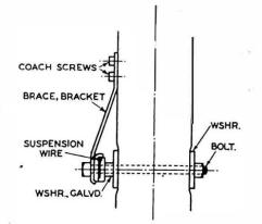
FIG. 4.-METHOD OF ATTACHMENT FOR SUSPENSION WIRE"
