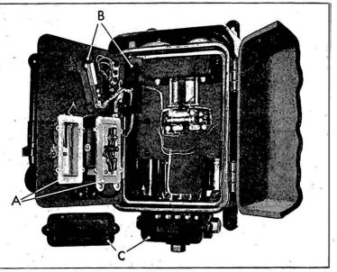
FIG. 4.—TELEPHONE NO. 153-INTERNAL LAYOUT.
