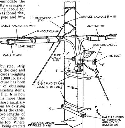
FIG. G .--- MOUNTING OF LOADING COIL CASE.
