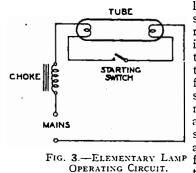
lamps it is necessary to have a current limiting device in the line, and due to the length of the tube, and to the fact that it is designed to work on mains voltage, an au tomatic starting switch is incorporated, the essential function of which is to assist in the pro-
