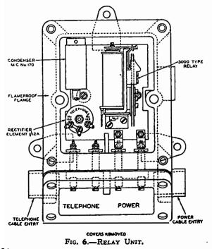
flameproof apparatus was desirable. As mentioned previously, no satisfactory flameproof loud sounding bell, suitable for operation on the standard telephone circuit, and by the normal ringing current, was available, and the only alternative was to provide some device similar to a relay switch which could be used to operate an electric supply mains device, of which several were available.
