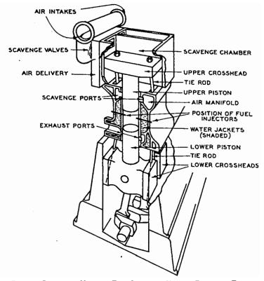
FIG. 2. SECTIONAL VIEW OF TWO CYLINDER UNIT OF FULLAGAR ENGINE.
