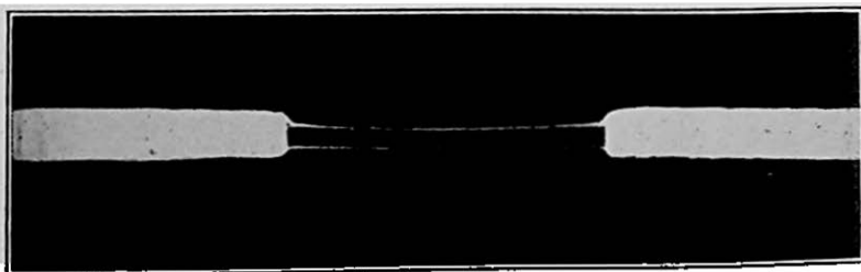
FIG. 2.—SAMPLE OF POLYTHENE AFTER COLD DRAWING.
