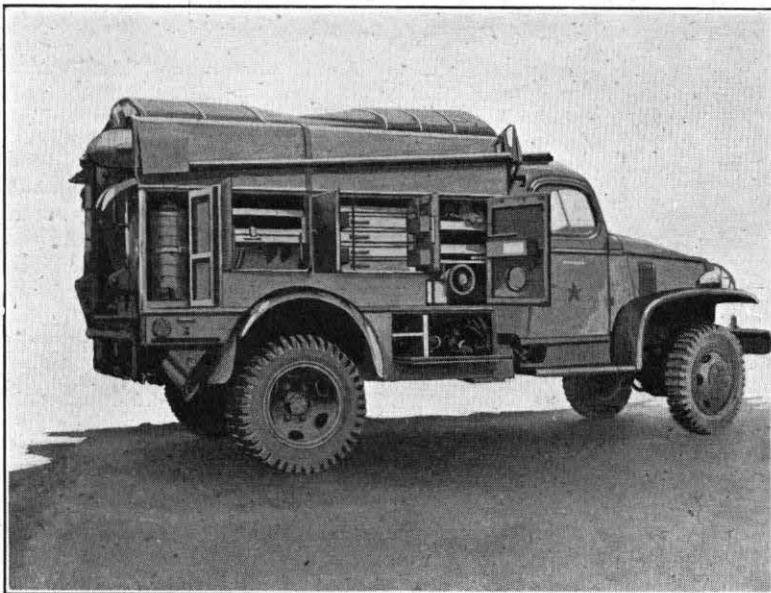
FIG. 3.—LINE CONSTRUCTION TRUCK.
