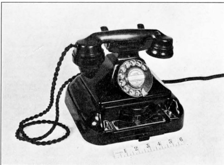
FIG. 1.—TELEPHONE NO. 248 WITH BELL SET NO. 39.
