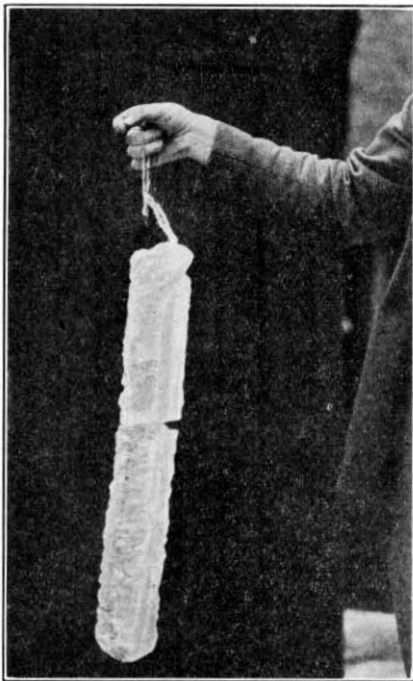
FIG. 1.—A TYPICAL ICE-COATED WIRE, WORCESTER.
