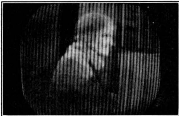
(e) Single-frequency noise, 500 kc/s approximately, bar pattern.
