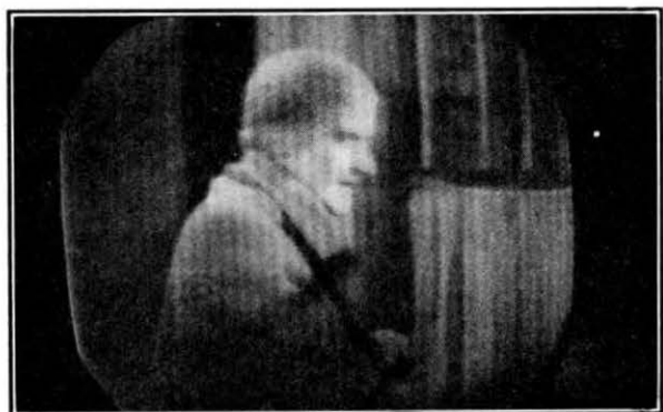
(f) Single-frequency noise, 500 kc/s approximately, mesh pattern.
