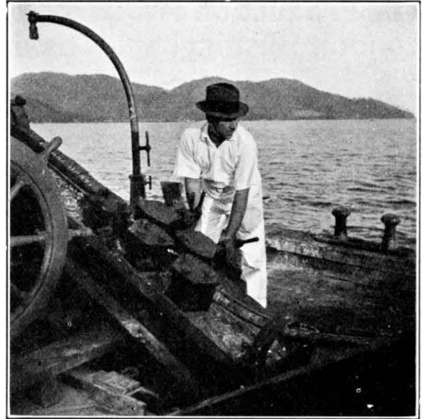
FIG. 7.—CABLE BRAKE IN OPERATION.
