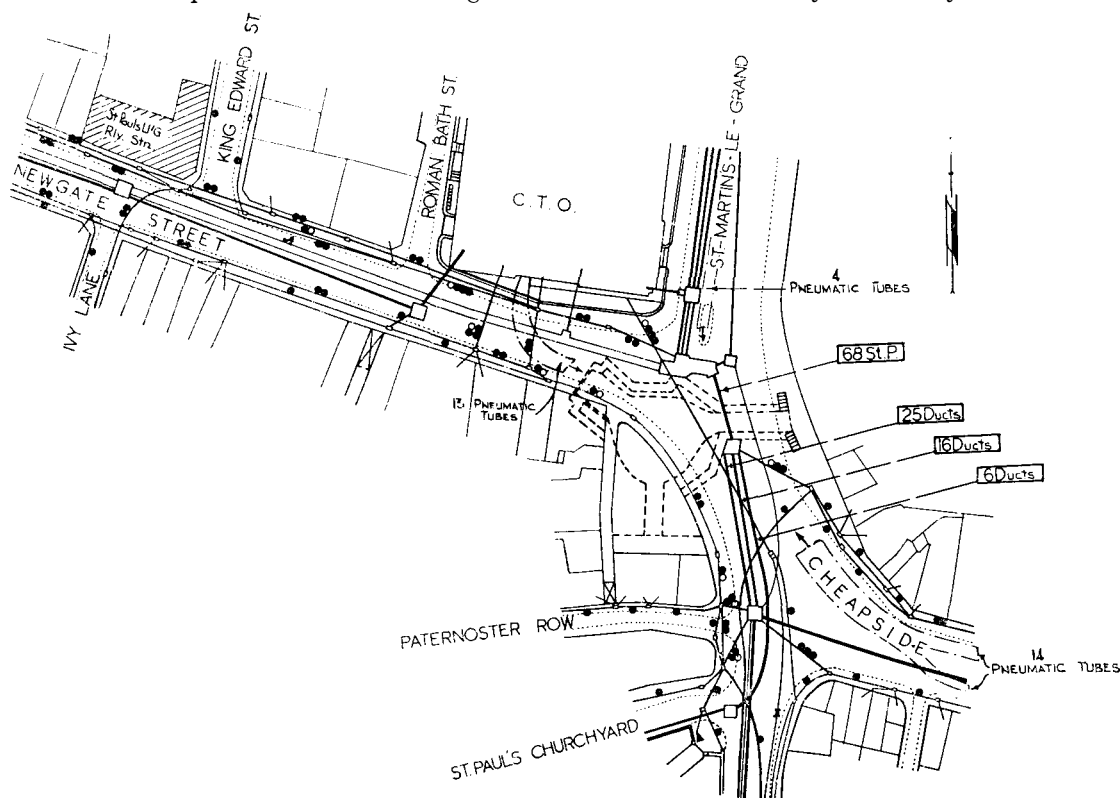
FIG. 1.—PLAN SHOWING POST OFFICE PLANT AFFECTED.
