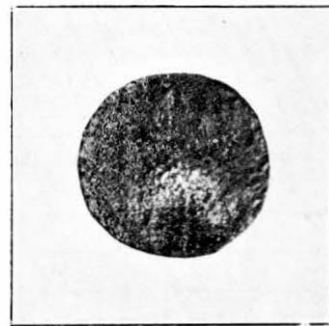
FIG. 5.—TYPICAL FATIGUE FAILURE.
