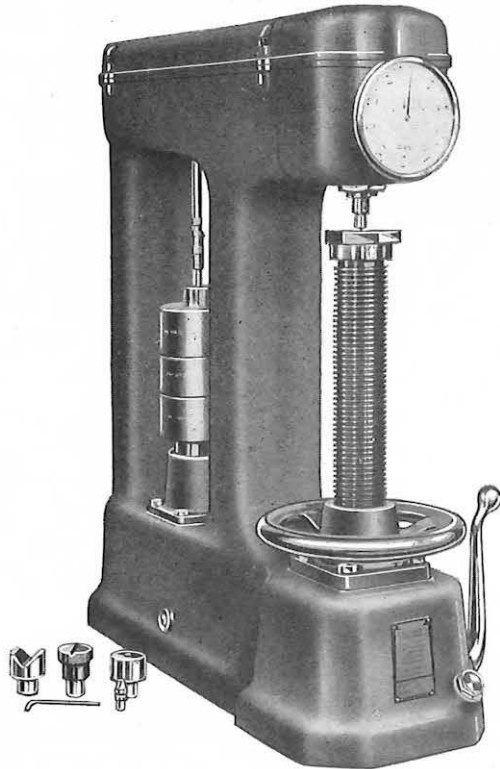
FIG. 1.—AVERY'S DIRECT READING HARDNESS TESTING MACHINE.
