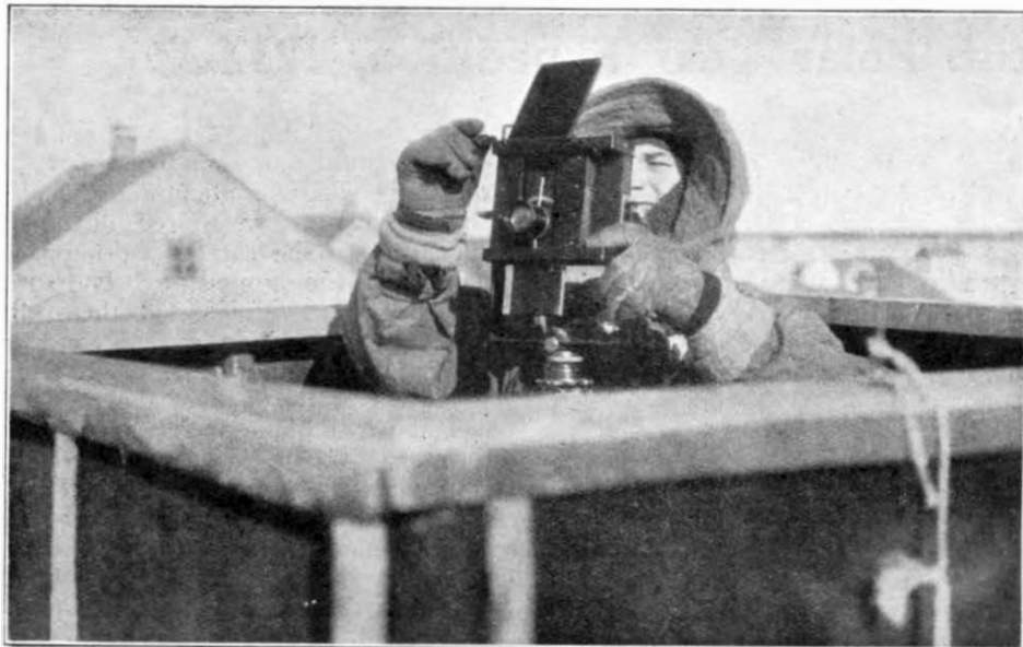
OPERATING THE AURORAL CAMERA INSIDE THE SHELTER. THE SLIDE CARRYING THE LENS CAN BE MOVED INTO SIX DIFFERENT POSITIONS RELATIVE TO THE PLATE, SO ALLOWING SIX EXPOSURES ON EACH PLATE TO SAVE TIME ON OCCASIONS OF QUICKLY CHANGING AURORA.
