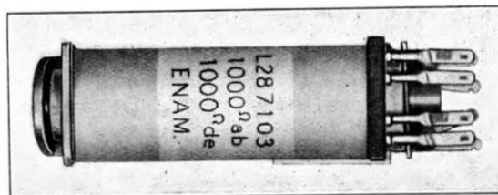
FIG. 5.—TYPICAL COIL MARKING.
