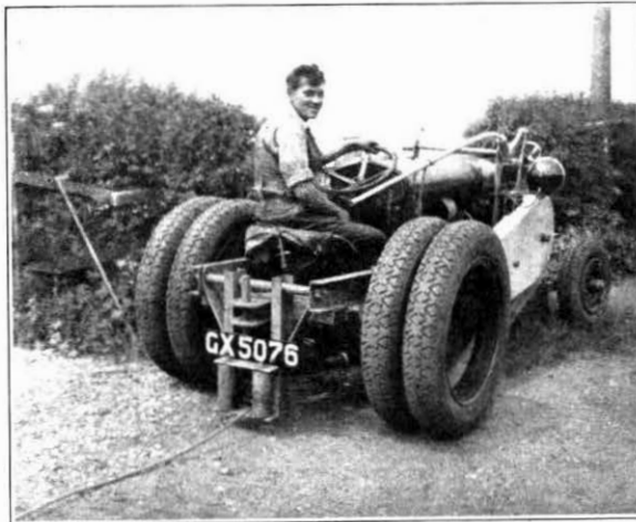
Fig. 2.—Rear view, showing steel Hawser and Guide Rollers.
