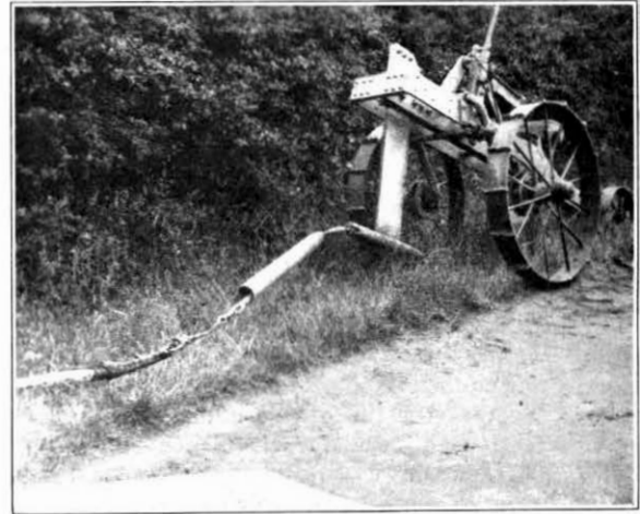
Fig. 4.—Mole Drainer, showing make off of cable, mechanical fuse and cylindrical cover for fuse with torpedo end.
