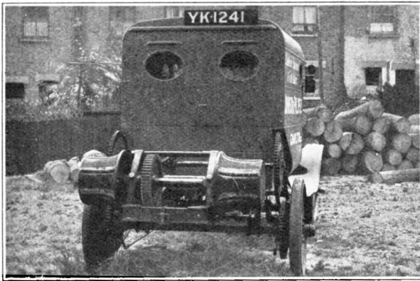
FIG. 3.—J. AND P. CABLING MACHINE.
