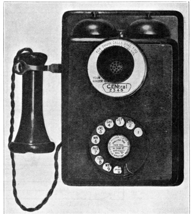
FIG. 10.—WALL TELEPHONE. MULTI-OFFICE AREAS.
