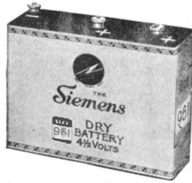
No. 961 L.T. Dry Battery for use with D.E. valves rated at 2.5 to 3 volts, current consumption 0.06 ampere.
