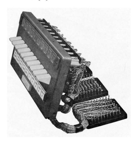
provided for the audible alarm so that it can be cut off, at will. The call is answered by moving the relative key up to a 'speak' position. The audible alarm then stops and the signal light goes out.
