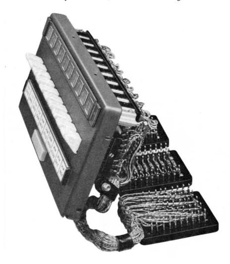
telephone exchanges, or on certain private circuits or extensions to a switchboard, outgoing calls are signalled by pressing a non-locking bar-switch beneath the identification strip on the unit, after selecting the circuit. The bar-switch is also used for operator recall and transfer facilities when the circuits on the unit are connected to a PBX. When any of these types of circuit is engaged on an outgoing call the signal lamps on all units to which it is connected will glow steadily.
