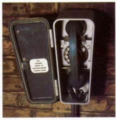
A wall-mounted telephone contained in a grey metal case, can be provided for use at outdoor locations. It may be used on exchange lines and switchboard extensions and associated with some plan arrangements. The hinged door is finished in blue and can be provided with a lock if required. The telephone, which contains an integral bell, may be fitted on a wall or to a pole. The case measures 318mm by 145mm by 168mm, and the total weight is 5 kg.
