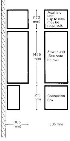
The above illustration shows the 4 + 18 size equipment. The 2 + 6 and 3 + 12 sizes differ in the height of the power unit which is 266mm and 355mm respectively.
