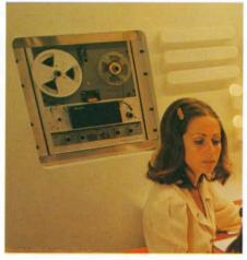
At most studios an audio tape recorder enables the conference to be recorded or it can be used to transmit pre-recorded messages.
