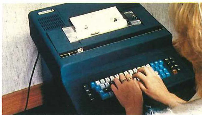
PUMA A fully electronic teleprinter using microprocessors to provide advanced facilities. It has its own memory.
