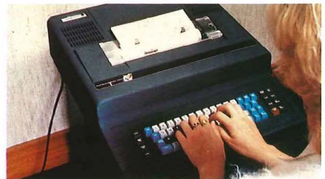
PUMA A fully electronic teletypewriter using microprocessors to provide advanced facilities. It has its own memory.
