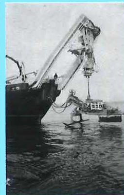
Cover: The laying of the world's first commercial undersea optical fibre cable between the UK and Belgium was scheduled for completion by the end of May. In the weeks leading up to the event extensive trials were held off Ramsgate with BTI's cableship Alert and its remotely controlled submersible Plough. (See page 43).
