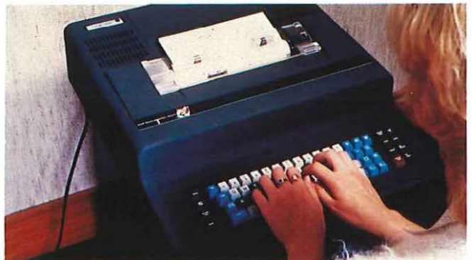
PUMA A fully electronic teleprinter using microprocessors to provide advanced facilities. It has its own memory.
