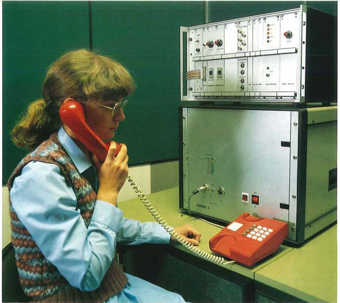
Expert in phonetics, Louise Helliker, checks that the equipment can recognise connected speech over a telephone line.
