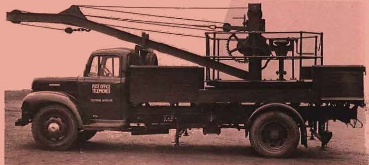
Above: Muscle-power not horse-power operated this 1951 crane lorry.
