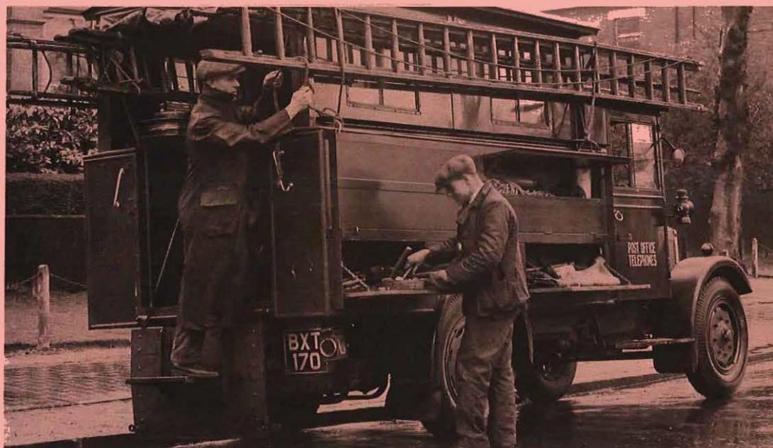
Right: An Albion 30cwt utility vehicle used by local line construction gangs in the 1930s. Note acetylene lamps.
