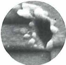
A view magnified 2,000 times of damage to a polysilicon input resistor caused by only 500 volts.
