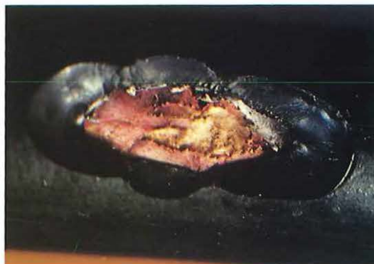
Although buried four feet underground, this fibre optic cable on a major trunk route was damaged because of its metallic moisture barrier.
