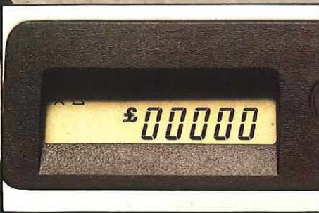
5 digit custom LCD displays call cost, accumulated charges and programming information.
