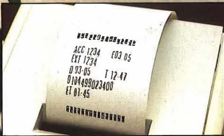
Integral micro thermal printer provides hard copy record either automatically or on demand.
