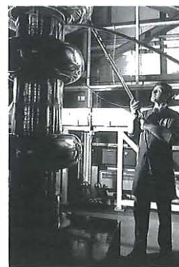
Cover: A high-voltage tester developed to check the stress levels of submarine cables proves a dramatic sight at British Telecom's Martlesham Research Laboratories. Pictured working on a cable for the proposed UK-Belgium link, technician Carlo D'Inverno uses an earthing wand to discharge the cable. The machine generates a DC potential of half a million volts.
