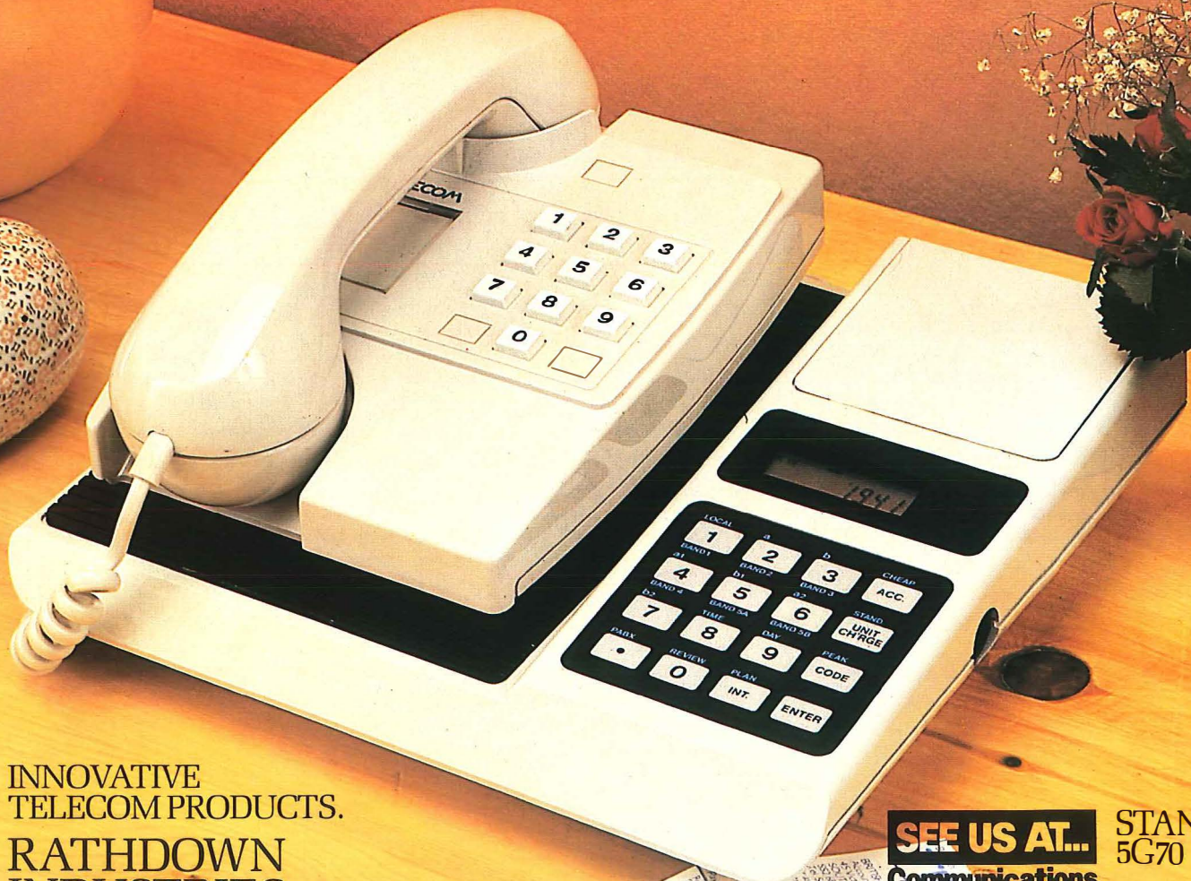
Simply plugs into any telephone line, PSTN or PABX; requires no exchange meter pulses.
