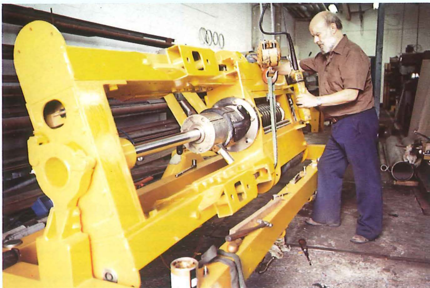
Below: Technical officer Bill Boothsby reassembles one of Marine Services' cut-and-hold grapnels following a major overhaul, including shot blasting and repainting. The grapnel was subsequently shipped to Geneva for display at Telcom 83.
