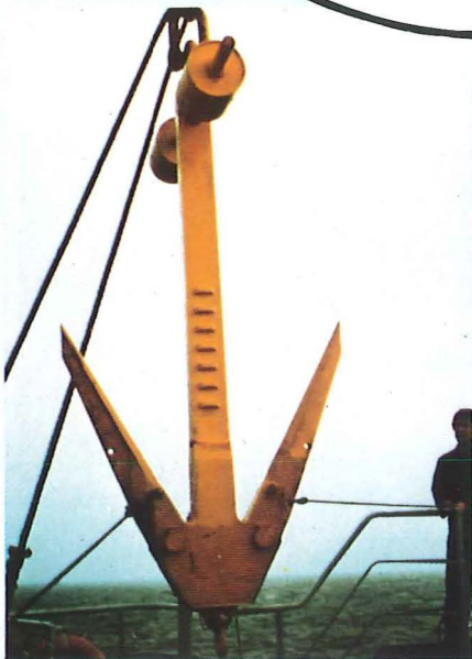
Below: Technical officer Bill Boothsby reassembles one of Marine Services' cut-and-hold grapnels following a major overhaul, including shot blasting and repainting. The grapnel was subsequently shipped to Geneva for display at Telcom 83.
