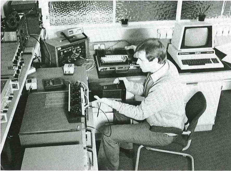
A laboratory used by British Telecom to evaluate manufacturers' equipment before its possible connection to the network.
