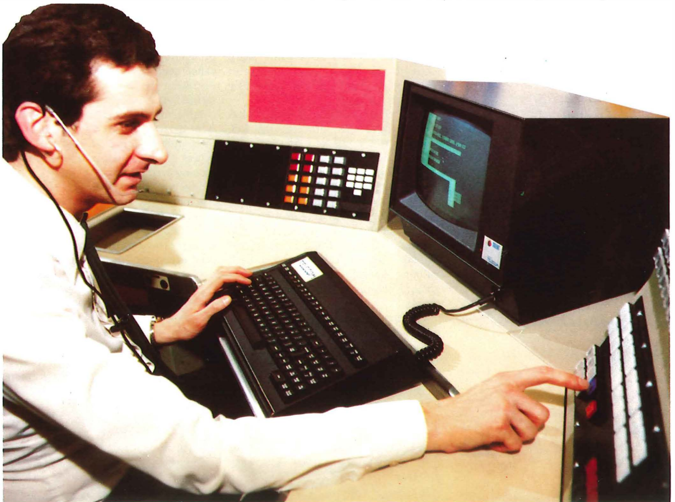
A control operator at a county fire brigade headquarters uses the Solent key panel to mobilise a remote fire station following an emergency call.
