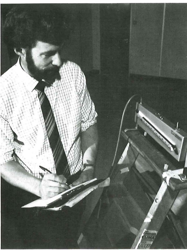
Guildford assistant executive engineer Alan Austin (left) checks the pressure drop across the adjustable air delivery slots using a manometer with the help of clerk of works technical officer Peter Woodward.
