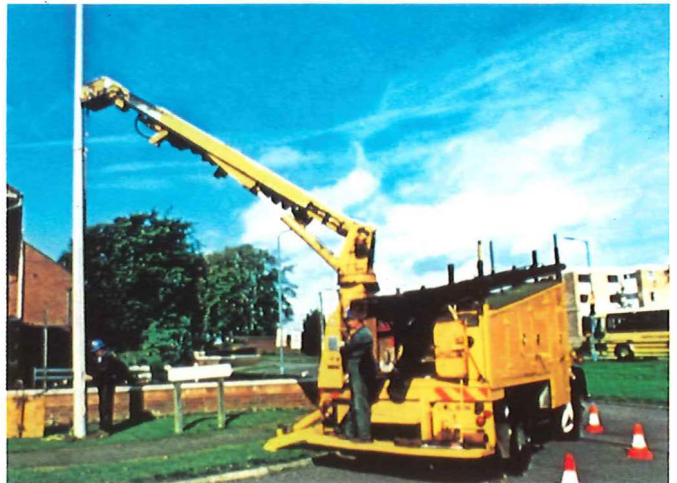
Above right: Rodding and light cabling vehicles are now widely used.
