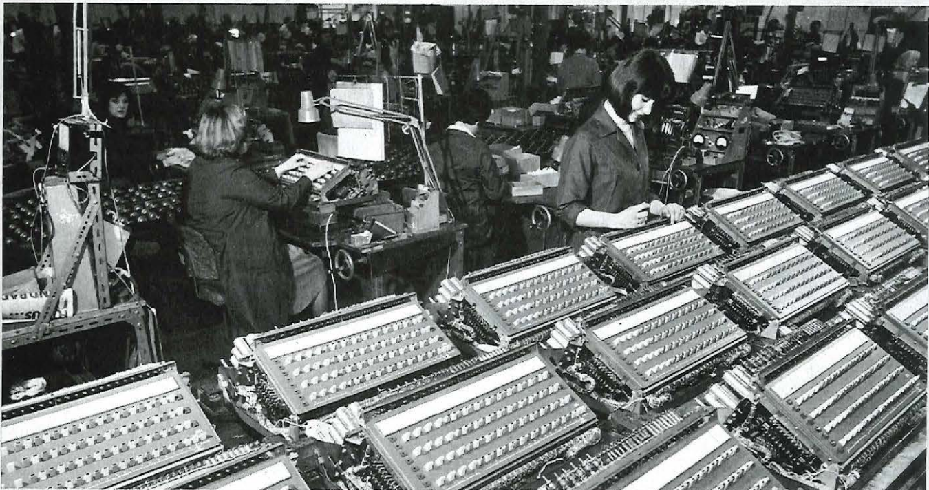
Staff at Enfield Factory refurbishing small private manual branch exchanges (PMBXs).
