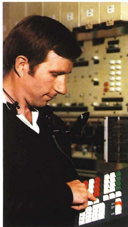
Technical officer Barry Cook tests a faulty console on the test rack which was formerly a prototype for international directory enquiry equipment.
