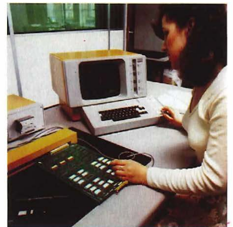
Tracing faults with Membrain automatic test equipment;
