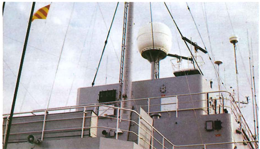
The Royal Fleet Auxiliary ship Olmeda is fitted with equipment necessary for communication by satellite.
