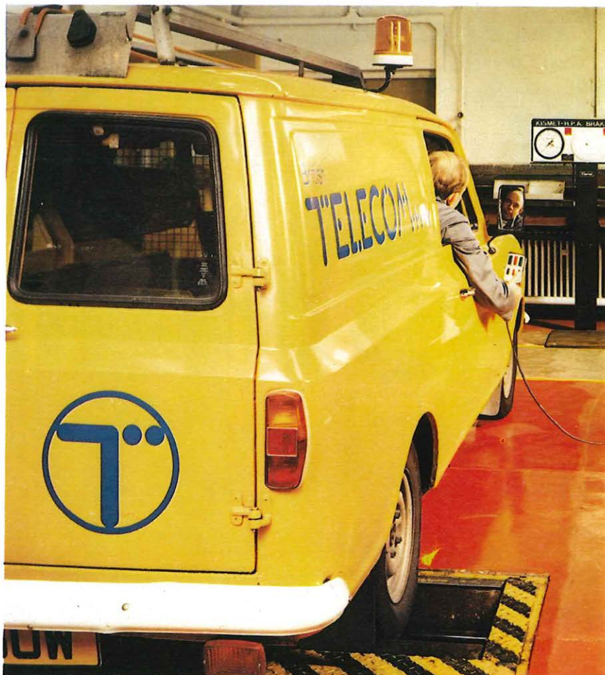
Brakes of a 7cwt van are checked using the roller brake tester.
