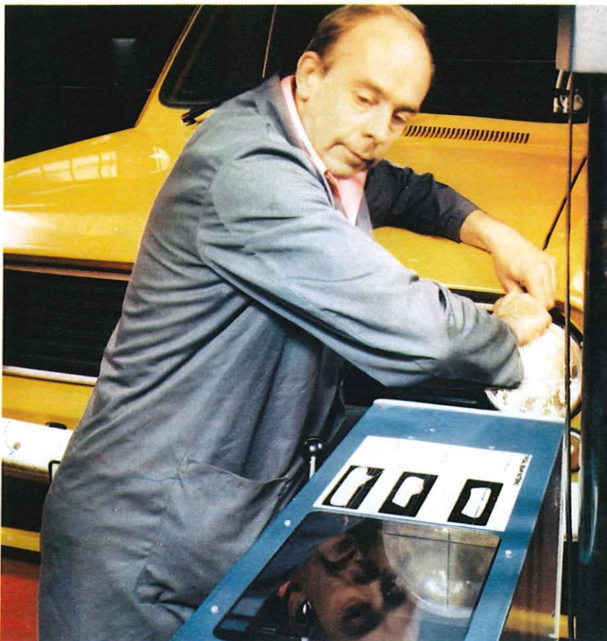
Headlights on a 7cwt van are aligned using a beamsetter.
