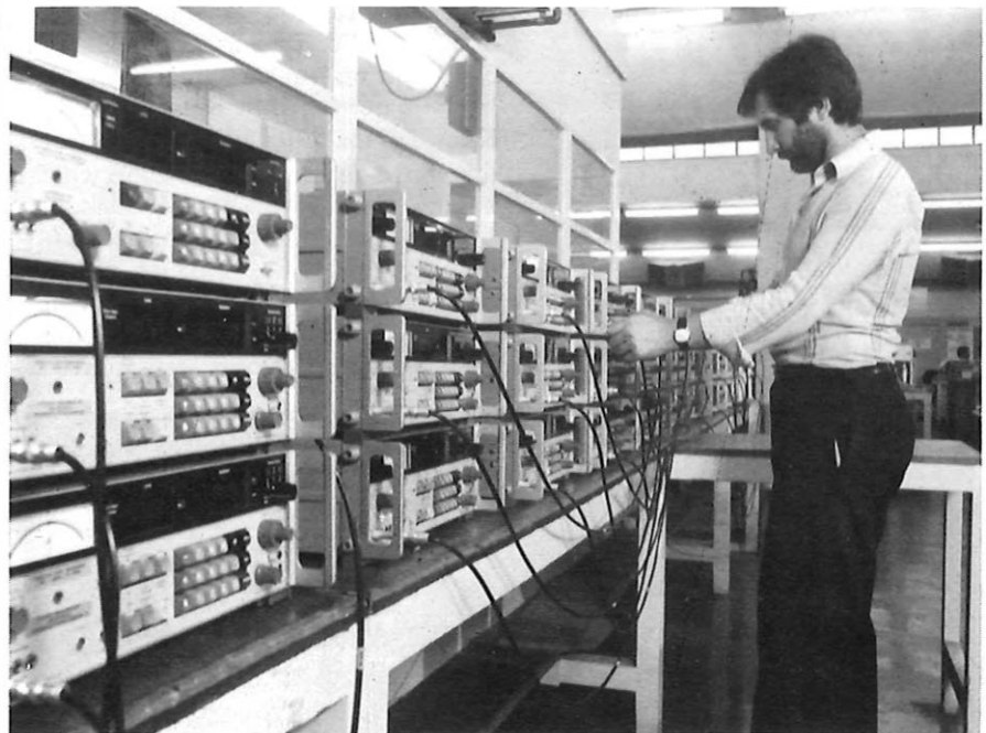
Selective level measuring sets undergo reliability approval checks at Marconi Instruments, St Albans.
