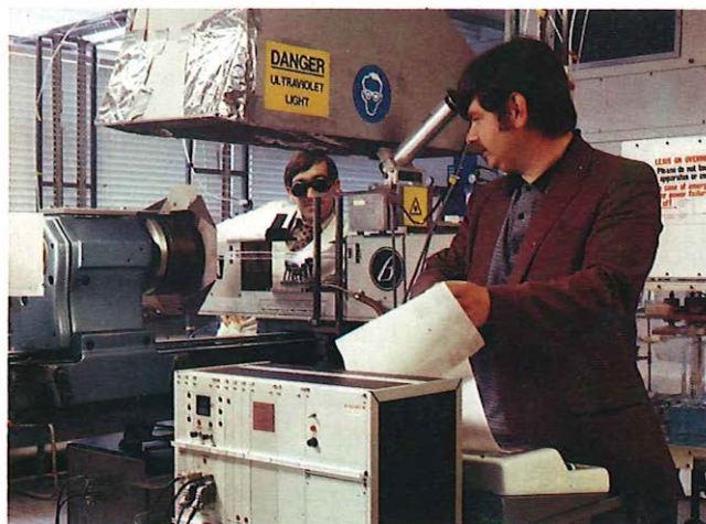
Dave Nelson, an AEE, checks the print out on the MSSS system which is being used as a precision temperature controller in the manufacture of low loss optical fibre at Martlesham.
