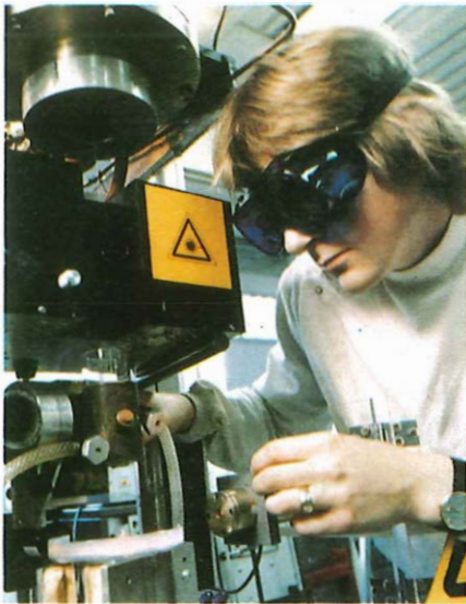
Martlesham technician David Colthorpe uses a laser to ensure that spun fibre is coated concentrically with silicon resin to prevent tiny cracks appearing on the surface.
