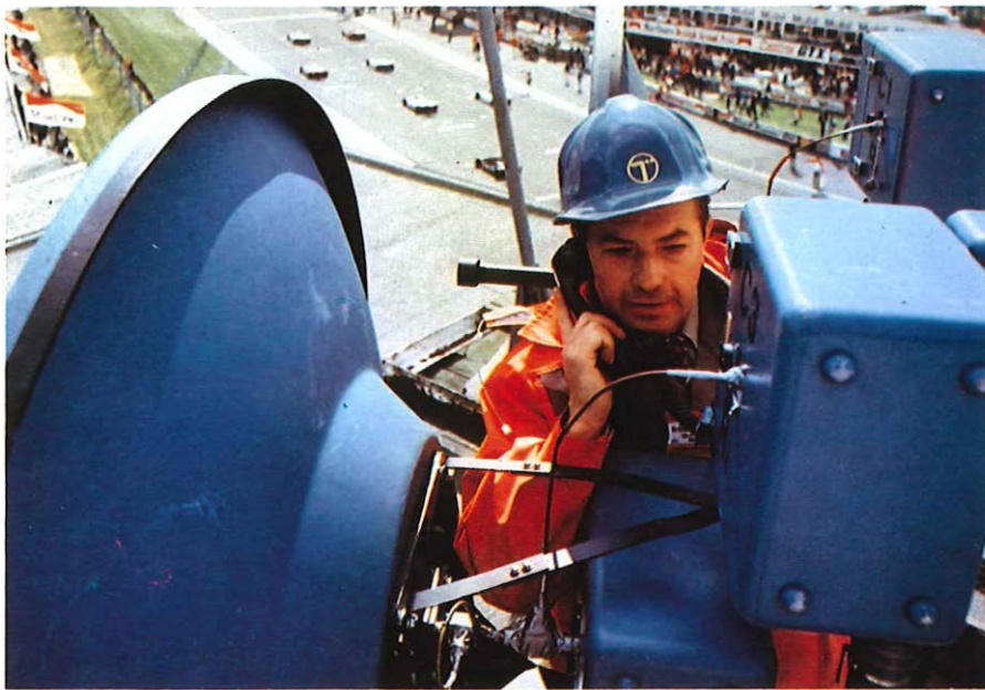
Above: As cars race by on the track engineer Michael Newbery checks the dish aerials used in the specially constructed microwave link at Silverstone.
