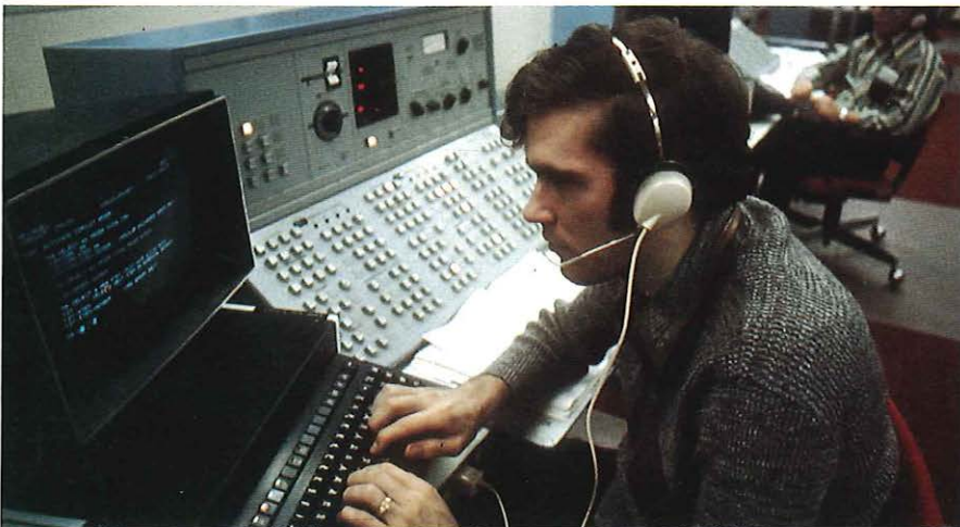
A Chicago-based AT&T technician working on an Electronic Switching System 4, a high-capacity, all-electronic toll switcher.
