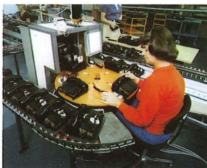
A stage in the manufacture of the new push-button Diavox telephone set which uses voice frequency signalling and has been developed with the modern AXE stored program control exchanges in mind.
