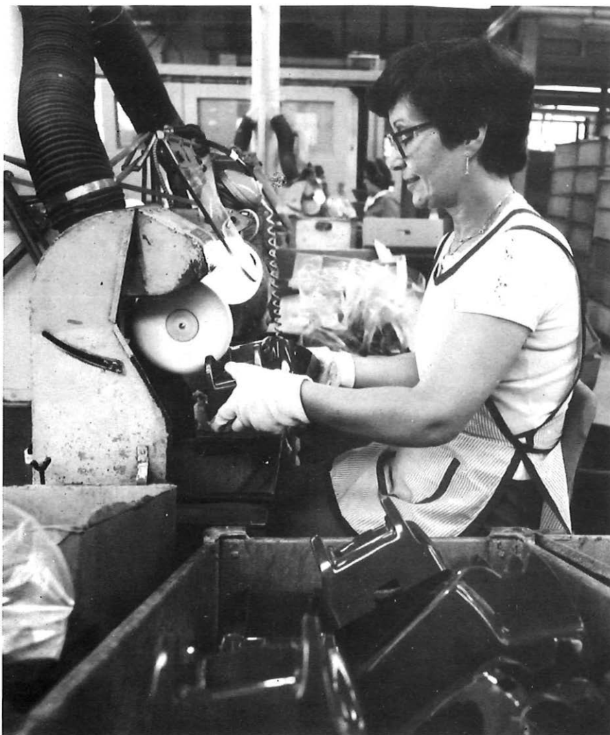
A wide range of plastic instrument mouldings are renovated at Cwmcarn. Here assistant factory technician Mrs Sylvia Cross begins polishing a binful of handsets – just a few of the tens of thousands of items handled at Cwmcarn each week.
