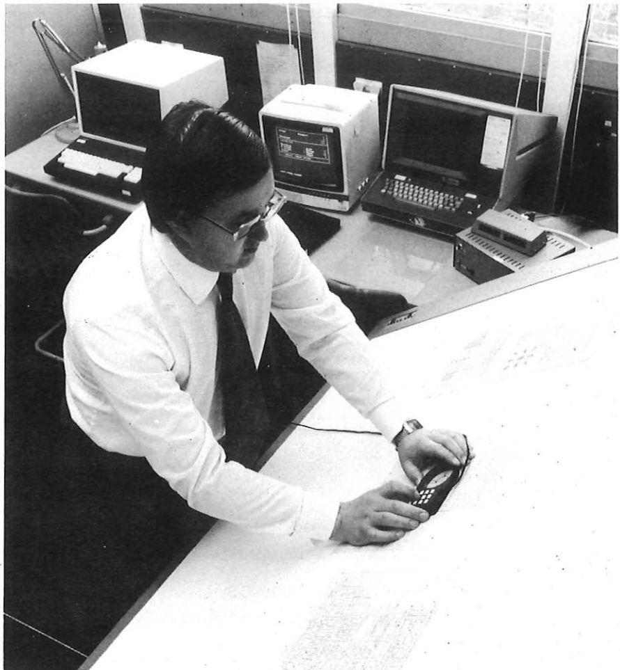
Peter Gill, AEE, uses a probe on the digitiser connected to the Poligon system to translate a layout drawing of a microchip output stage into data which can then be used for further computer processing.
