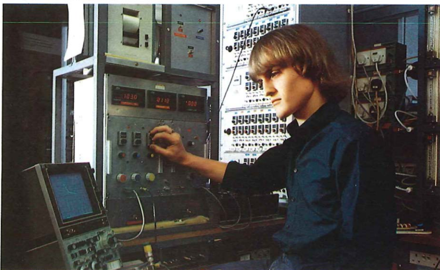
Third year TTA Richard Prodger uses an oscilloscope to check pulsed light output from a laser.
