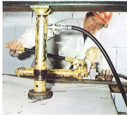
A concrete manhole cover is put under pressure at Smallford to determine its breaking point.
