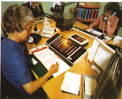
The new A345 electronic PBX which can serve between 500 and 7,000 extensions.
